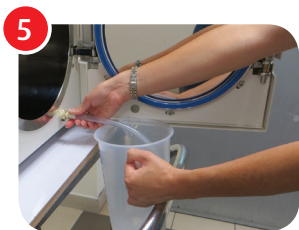
5 At the end of the cycle, open the door and drain the entire contents of the water reservoir.
